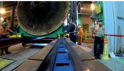
Standout features of the LP350 system include a low-maintenance graphite-steel slide surface, and a ratchet track design, allowing the push cylinders to automatically reset at the end of each stroke.
