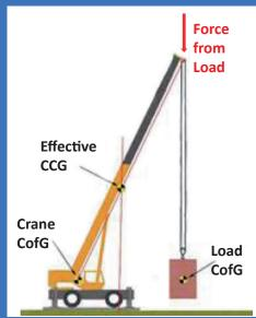
combined center of gravity of the crane and the load, to determine relative stability.
